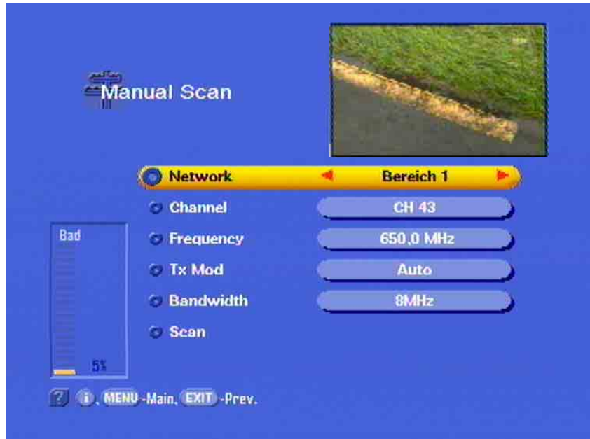
Picture above: Correct network, wrong channel, wrong frequency Picture below: Correct network, correct channel, correct frequency, Signal display: 'Good'
